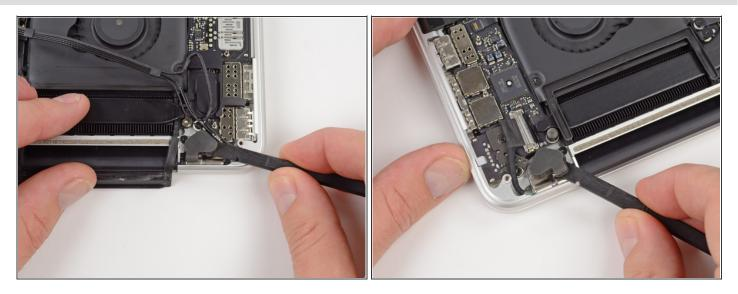
• Use the flat end of a spudger to pry off the two rubber hinge covers, one from each end of the device.
